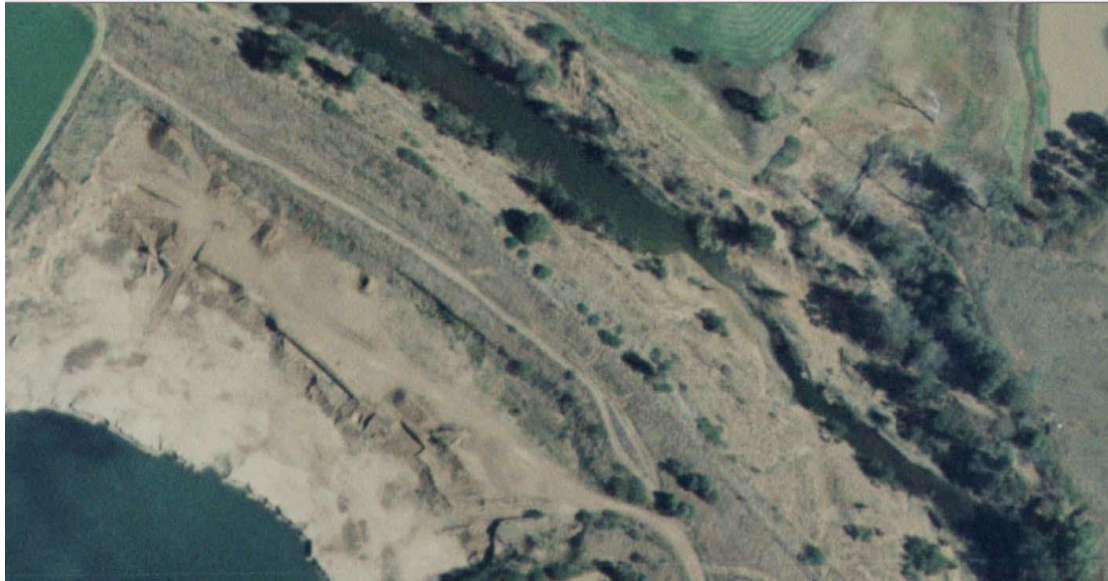
'Enlargement of 1997 air photo showing western levee – note no bunds either side of the access track.
